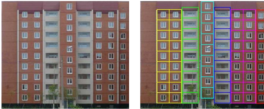
Figure 1: Input rectified image of building's facade (left) and automatically recognized structure, presented as a set of non-overlapping grids of similar windows (right).
