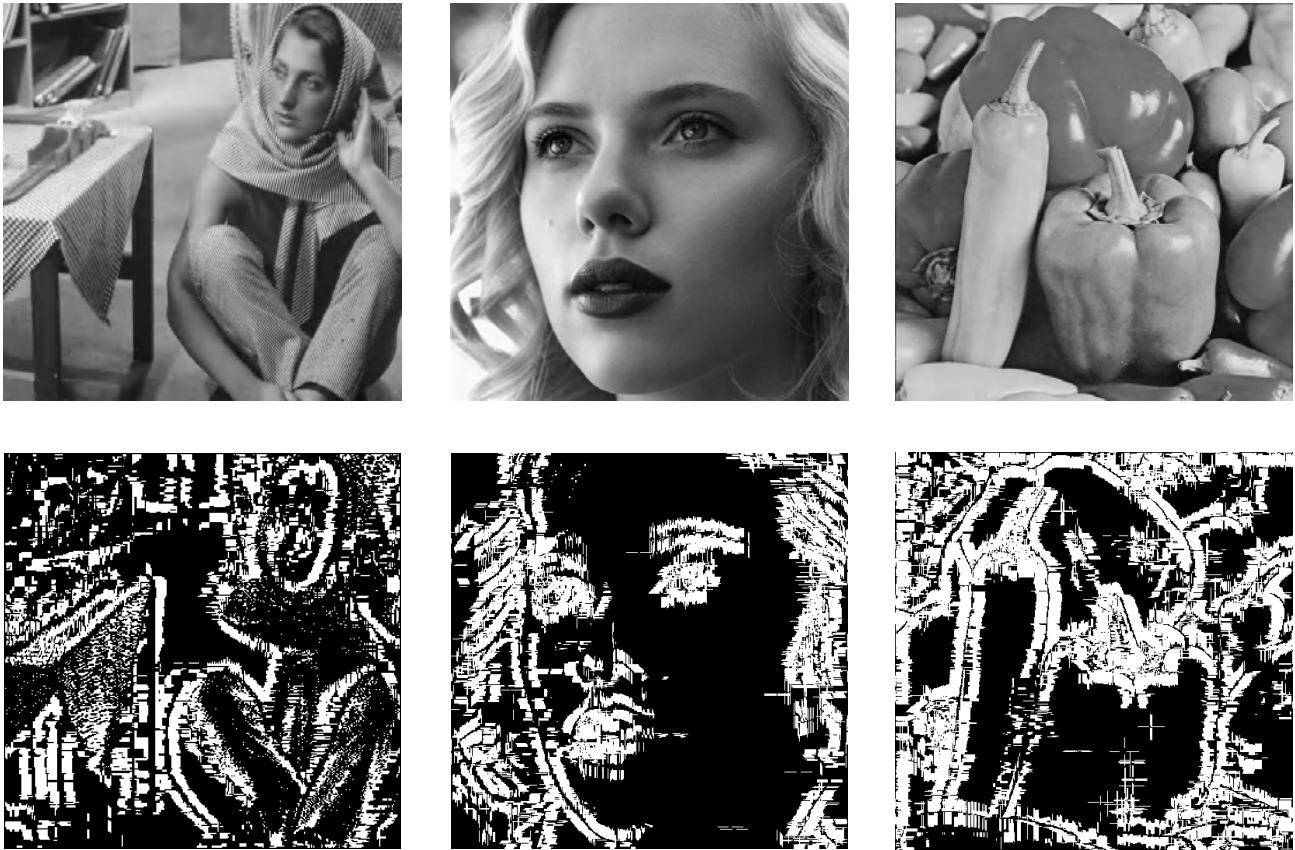
Fig. 2. Ringing maps for compressed test images (CR=17) “Barbara” (left), Scarlett (center), Peppers (right)
