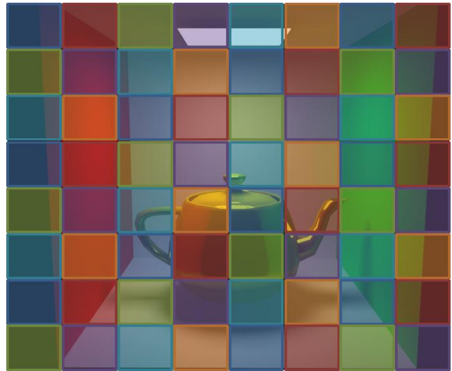
Figure 4. Screen divided into blocks. Blocks of the same color are processed by the same thread block
