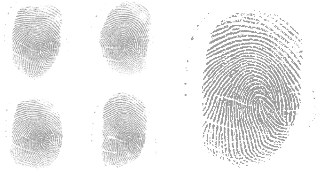
Figure 4: Deformation averaging (undeformed image is on the right)
