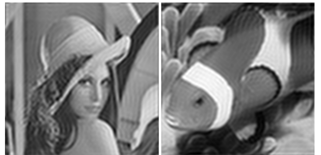
Figure 7: Input images with artificially added ringing artifact using high frequency data cut-off, first 1/8 coefficients of Fourier series were retained.
