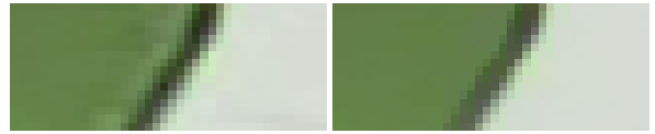
Figure 16: Blind image deringing. Left image: original image with ringing effect, R_E = 1.40 . Right image: the result of automatic deringing with ringing level control, R_E = 1.18 .
