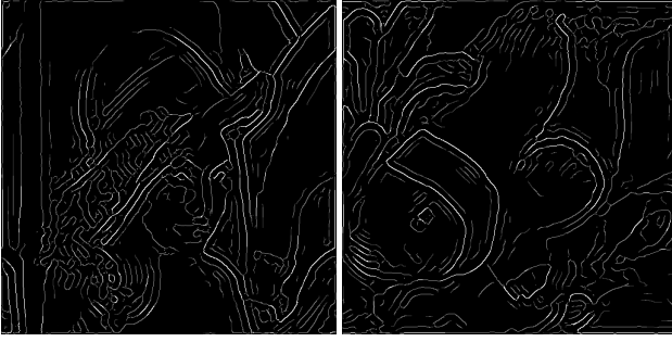
Figure 8: Results of Canny edge detector with \sigma = 1 to estimate ringing quasiperiod d for the input images from Fig. 7. White edges are important edges with high gradient value. Grey edges are edges with lower gradient values. Both grey and white edges are used for skeletonization, but only white edges will be used for basic edge selection.
