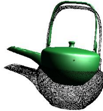
Figure 7: Point data set used for reverse construction (black) and an intermediate shape during the fitting process (green).
