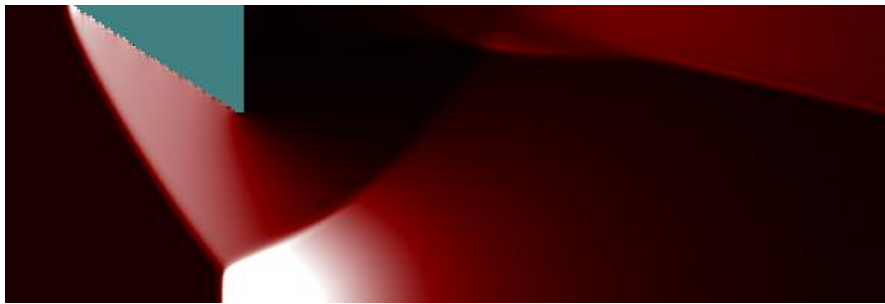
Fig. 2 Pressure Distribution for Supersonic Flow Around a Wedge with Mach Reflection
