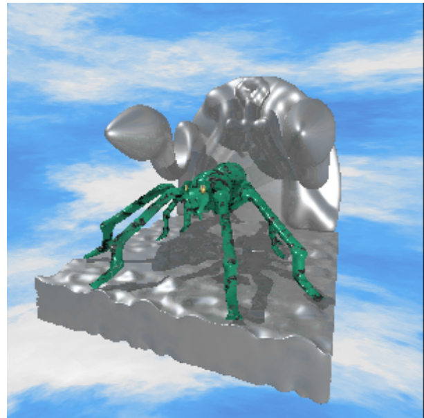
Figure 14: 3D solid modelled by building a tree with simple primitives and sculpted object using BSpline volumes.
