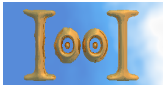
Figure 6: Modelling in a high resolution leads to some swellings. A multiresolution solves this problem.
